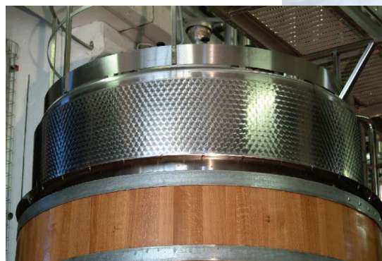
Stainless steel bonded to oak, a fundamental aspect of new Banfi fermenters.
