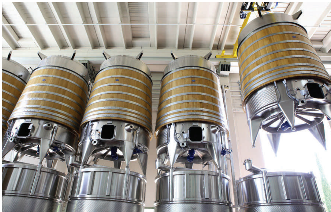
Composite fermenters being positioned atop storage tanks at Castello Banfi winery
